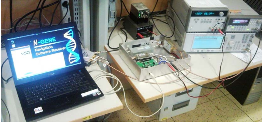
Fig. 3. Picture of the experimental setup (including the laptop for the raw data storage, the discrete component front-end, the power supply and the local oscillators) [own photo]
