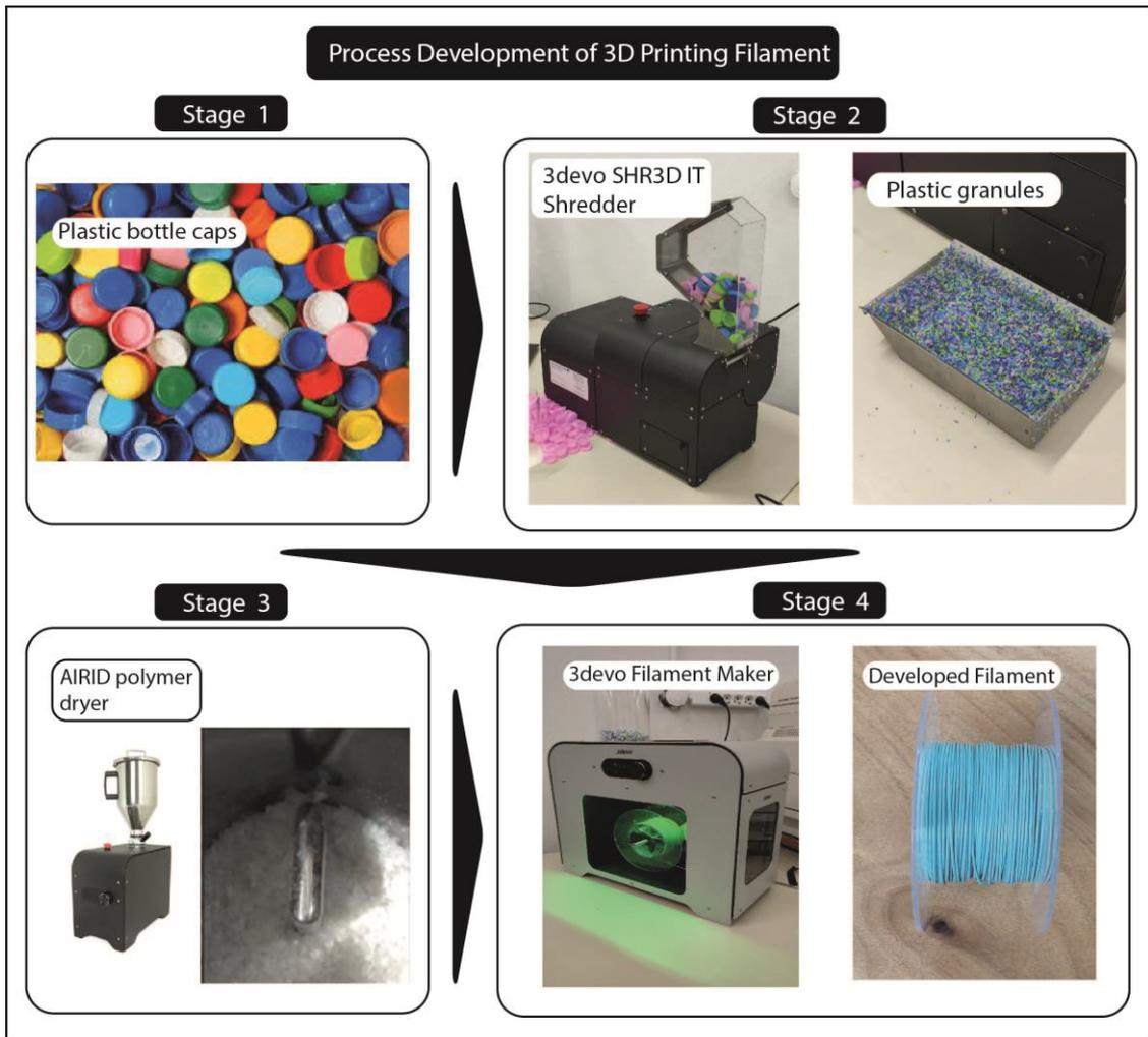
Figure 1: Manufacturing process 3D printing filament.
