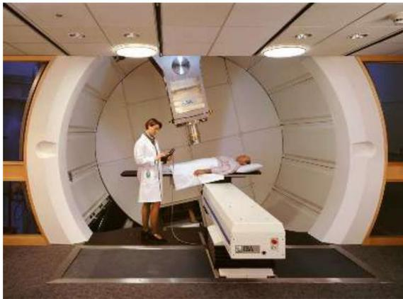
**Figure 18:** Gantry Treatment Room of the IBA Proton Therapy System.
