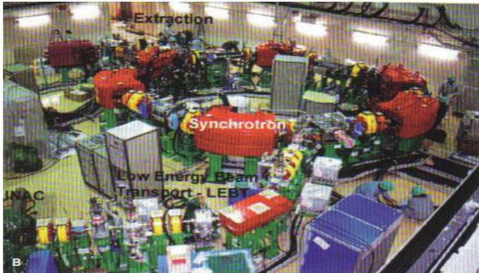
**Figure 20:** A view of Proton Synchrotron of 70 –250 MeV, [36].
