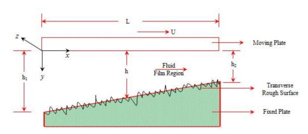
Figure 1. Configuration of the bearing system (Patel and Deheri, 2013a)
