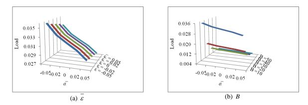
Figure 6. Profile of load bearing capacity with regards to  $\overline{\alpha}$
