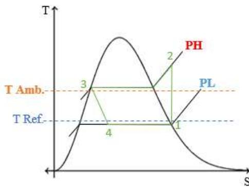
**Figure 1** Diagram of the simple compression refrigeration cycle
