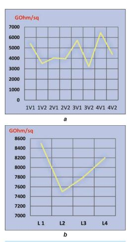
Fig. 3. Surface resistivity for: a - textile materials, b - leathers
