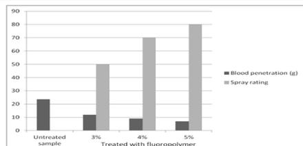
**Figure 1 Effect of fluoro polymer treatment on blood repellency**
