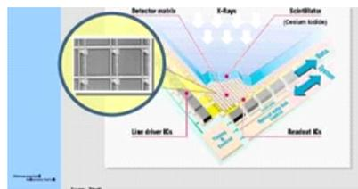
**Figure 1. Flat detector technology is based on CsI and an active pixel matrix of amorphous silicon.**
