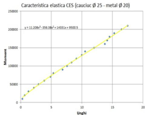
Figure 4: experimental characteristic of the coupling
