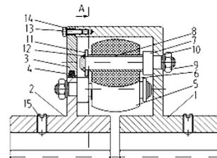
**Figure 2: longitudinal section of the clutches ling with metal and rubber rollers**
