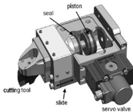
**Figure 4: Actuator device (HSK tool holder not shown).**<sup>[4]</sup>
