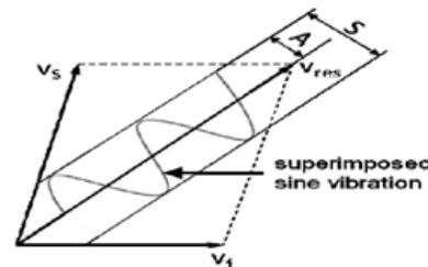
**Figure 2: Velocities (v), amplitude (A), peak-to-peak value (S) and superimposed sine vibration.<sup>[4]</sup>**
