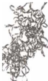
**Figure no. 6 : Chips generated by conventional turning**<sup>[6]</sup>
