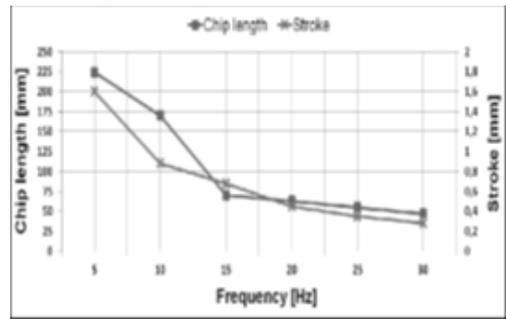
**Figure no. 7: Chip length in dependency on applied frequency** [4]
