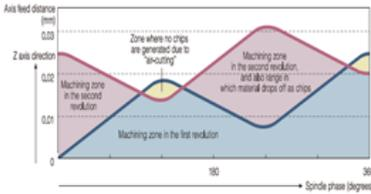
**Fig. 3 Feed distance per spindle revolution.**
