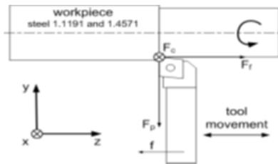
**Figure 1: Tool movement and forces during vibration<sup>[4]</sup>**
