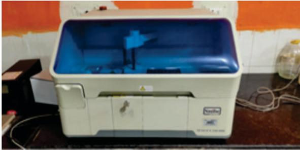
**Figure: Snibe Maglumi 800 for D-Dimer, IL-6, Ferritin, TROPONIN-I, PROCALCITONIN**
