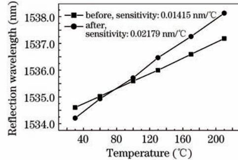
Fig. 7. Reflection wavelength versus temperature for the FBG sensor before and after metal coating and embedding.
