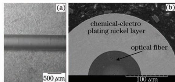
Fig. 3. Electroplating results with nickel conductive layer under optimum conditions. (a) The optical fiber after plating; (b) radial cross-section of the coated fiber.
