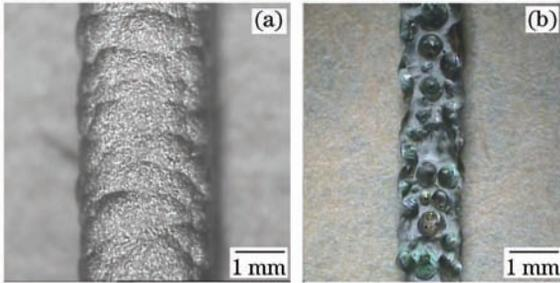
Fig. 5. Electroplating results under improper conditions. (a) Coarse characteristics; (b) porous characteristics.
