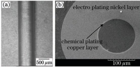
Fig. 4. Electroplating results with copper conductive layer under optimum conditions. (a) The optical fibre after plating; (b) radial cross-section of the coated fiber.
