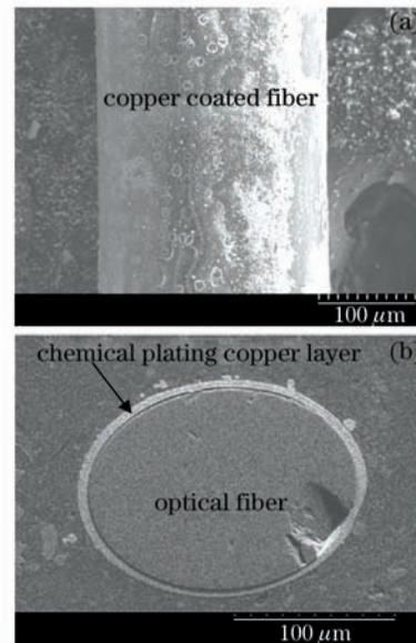
Fig. 2. SEM images of chemical plating copper conductive layer under optimum conditions. (a) The optical fiber after chemical plating; (b) radial cross-section of the coated fiber.
