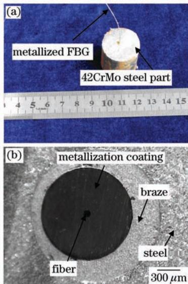
Fig. 6. (a) FBG embedded in a 42CrMo part; (b) radial cross-section of the part.
