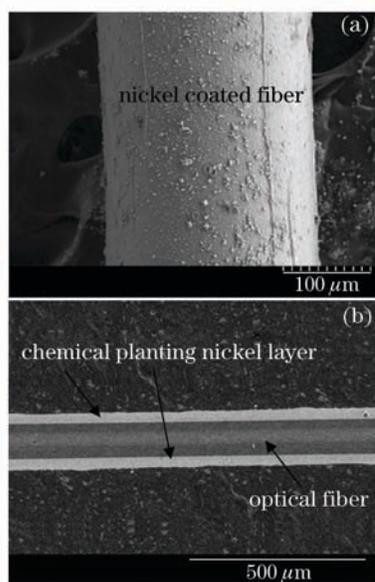
Fig. 1. SEM images of chemical plating nickel conductive layer under optimum conditions. (a) The optical fiber after chemical plating; (b) axial cross-section of the coated fiber.
