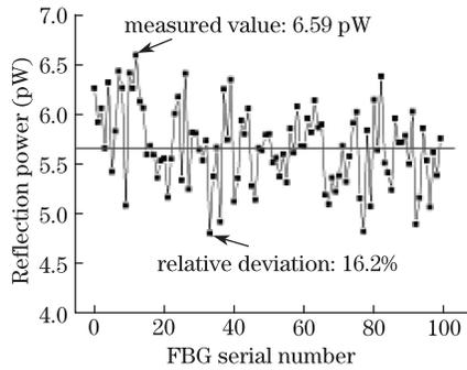
Fig. 7. Single FBG reflection power of 100 FBGs in array A investigated using a light source power of 2.5 nW at 1303.638 nm.
