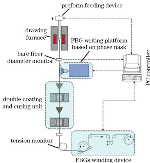
Fig. 1. Diagram of the on-line writing FBG system.
