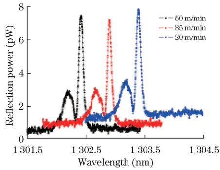
Fig. 4. Reflection spectra of three FBGs written at different speeds.
