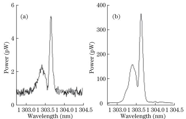
Fig. 3. Reflection spectra of array A and its single FBG, investigated with a light source power of 2.5 nW at 1303.638 nm.
