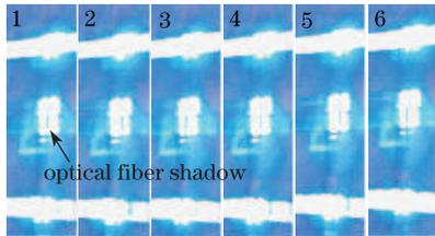
Fig. 8. Six images of the diffraction spot taken at a drawing speed of 12 m/min, average drawing tension of 38.2 g, and laser frequency of 50 Hz.
