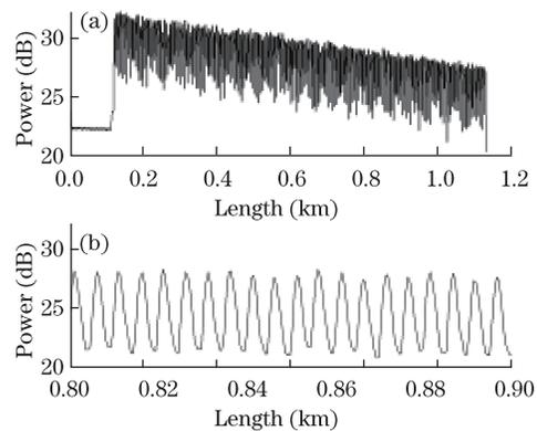
Fig. 2. (a) OTDR fragment from 200 FBGs of array A; (b) local enlargement between 0.8 and 0.9 km.
