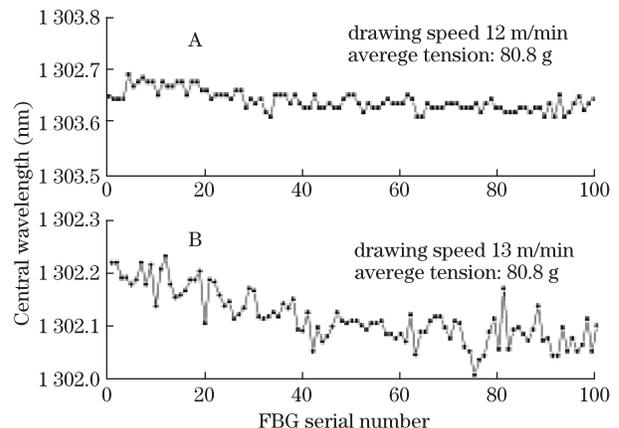
Fig. 6. Central wavelength distribution of successive 100 FBGs in array A and array B.
