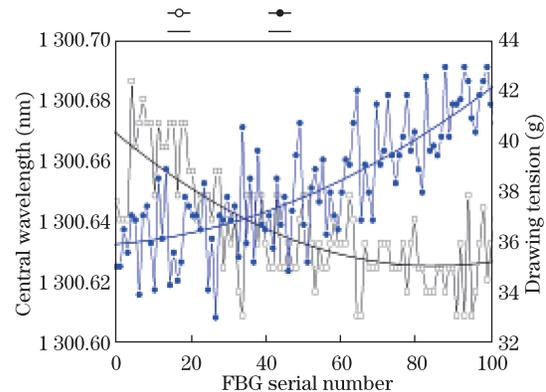
Fig. 5. Central wavelength and drawing tension traces of successive 100 FBGs in array A.
