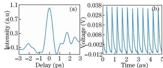
Fig. 6. Temporal characteristics of the mode-locked laser: (a) autocorrelation trace of the stretched pulse mode-locked laser and (b) pulse train with repetition rate of 2.38 MHz.
