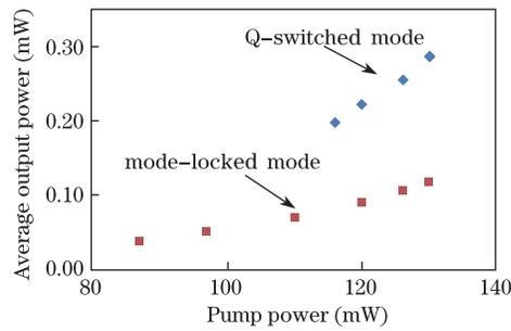
Fig. 7. Average output power against pump power for Q-switched and mode-locked EDFL.
