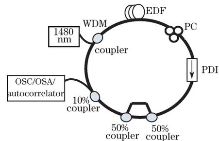
Fig. 1. Experimental set-up of the proposed switchable dual-function EDFL.
