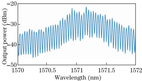
Fig. 4. Enlarged figure of the output spectrum of the Q-switched EDFL showing a comb spectrum.
