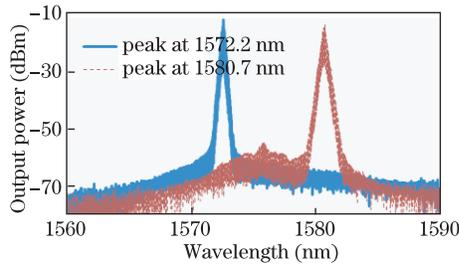
Fig. 2. Output spectrum of the EDFL at two different PC settings when the 1480-nm pump is fixed at 130 mW.
