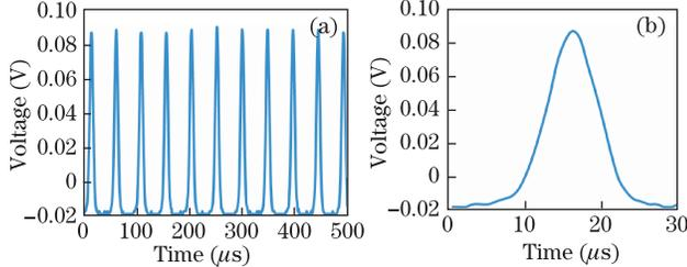
Fig. 3. Pulsing behavior of the proposed Q-switched EDFL: (a) pulse train showing a repetition rate of 21.2 kHz and (b) single-pulse envelope showing a pulse width of 7.7  $\mu$ s.
