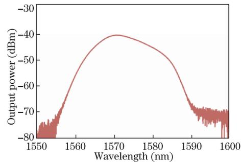
Fig. 5. Optical spectrum of the mode-locked fiber laser at pump power of 130 mW.
