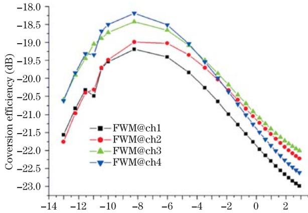
Fig. 5. Conversion efficiency of four channels at different pump signal powers.
