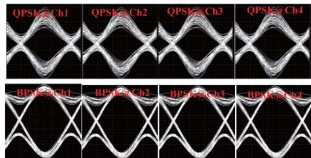
Fig. 8. Demodulated eye diagrams of converted BPSK signals for parallel four channels.
