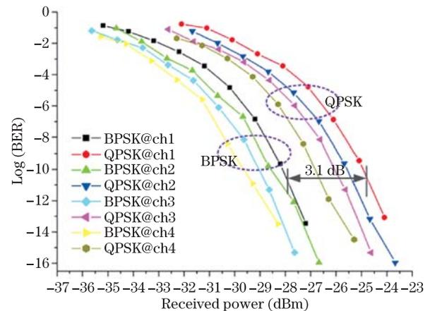
Fig. 7. Measured BER versus received power for four QPSK and BPSK signals.
