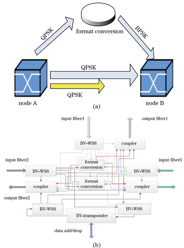
Fig. 1. (a) Illustration of an elementary two-node flexible-bandwidth network; (b) CDCG multi-degree ROADMs configuration based on format conversion. BV: bandwidth variable.
