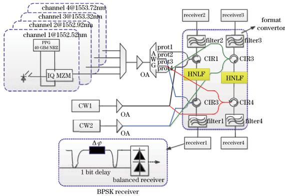
Fig. 3. Simulation setup for parallel four channels QPSK signals format conversion. CIR: circulator; OA: optical amplifier; PPG: programmable pulse generator.
