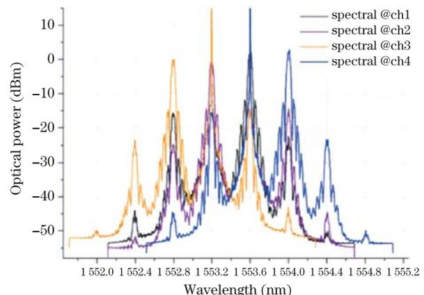
Fig. 4. Measured optical spectrum after HNLF in the format conversion simulation from QPSK to BPSK.
