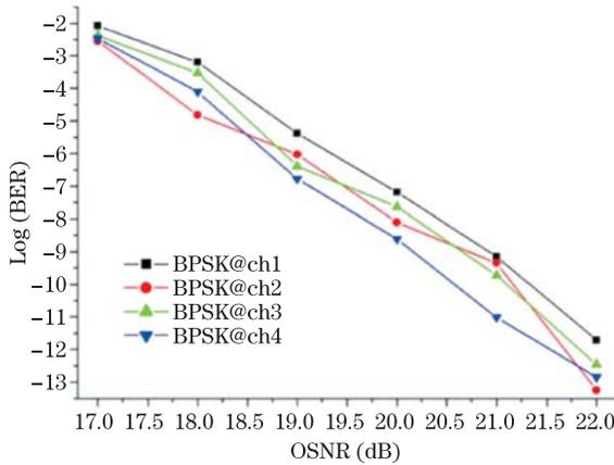
Fig. 6. Received BER versus input OSNR for four received BPSK signals.
