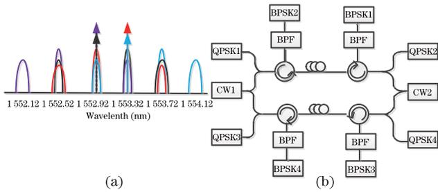
Fig. 2. (a) Wavelength position and (b) operation principle of the proposed parallel four channels format conversion system. BPF: bandpass filter.
