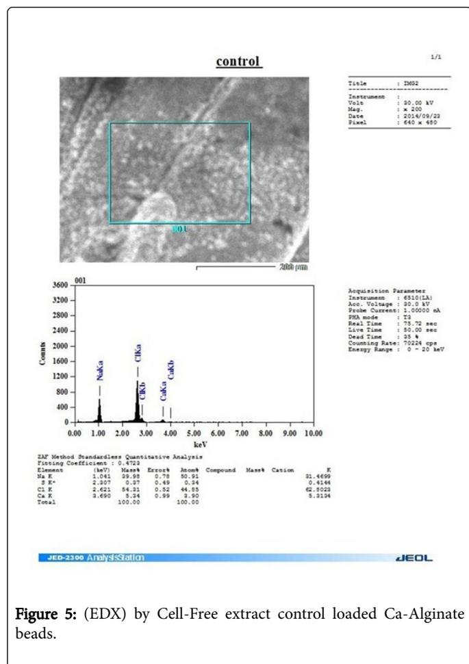
Figure 5: (EDX) by Cell-Free extract control loaded Ca-Alginate beads.
