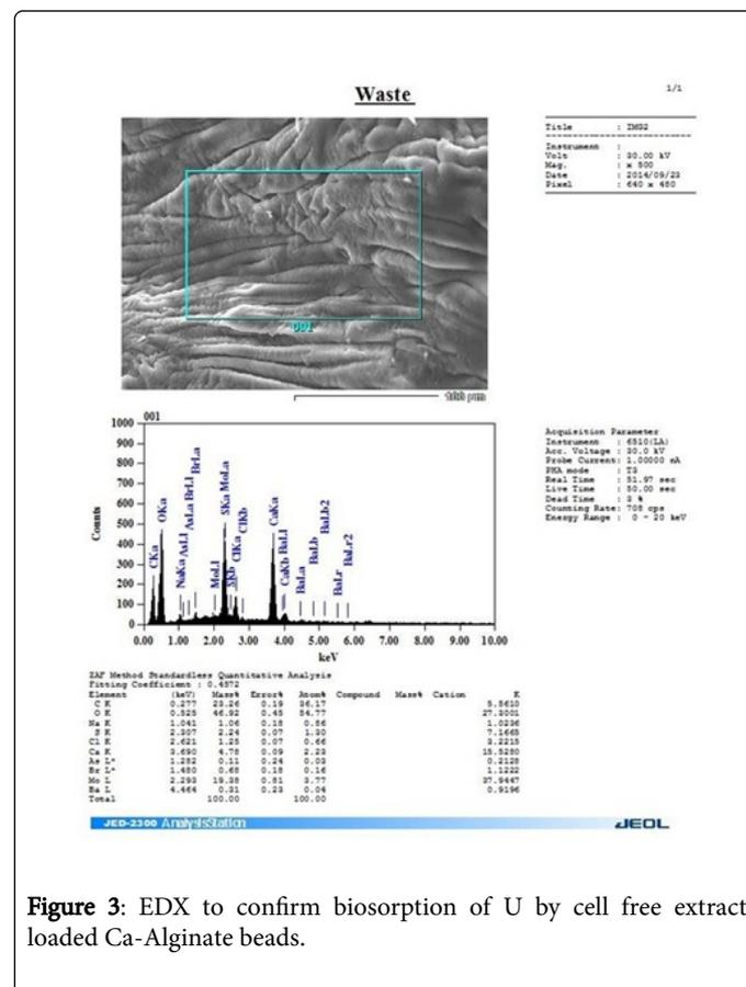
**Figure 3:** EDX to confirm biosorption of U by cell free extract loaded Ca-Alginate beads.
