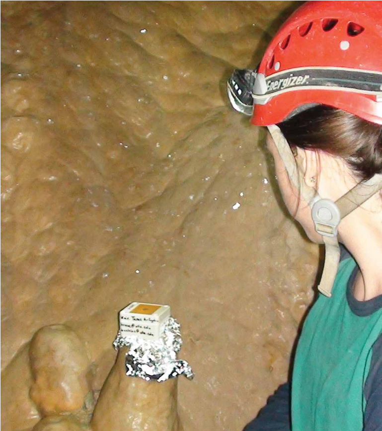
Figure 5. Set-up of Stalagmite monitoring station SM-4; temporary platforms for Stalagmite drip loggers were built with aluminum foil onto actively-growing stalagmites for the study duration.
