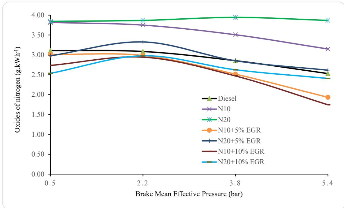
Fig. 9: Changes in oxides of nitrogen with BMEP.
