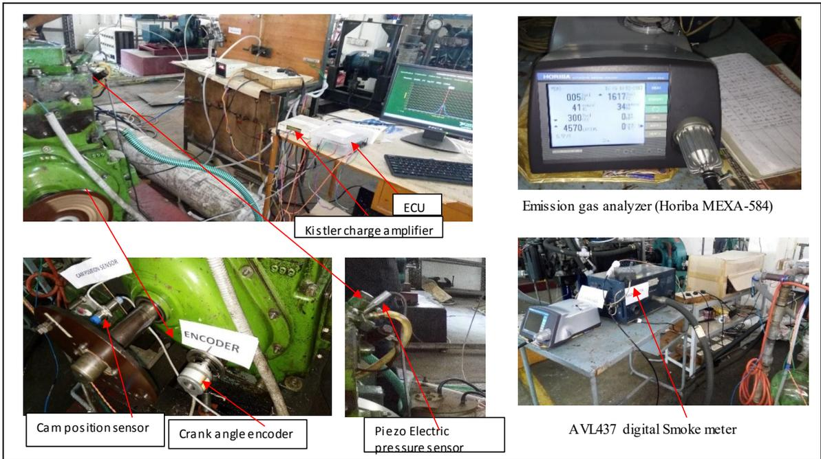
Fig. 3: Experimental setup – Photo.
