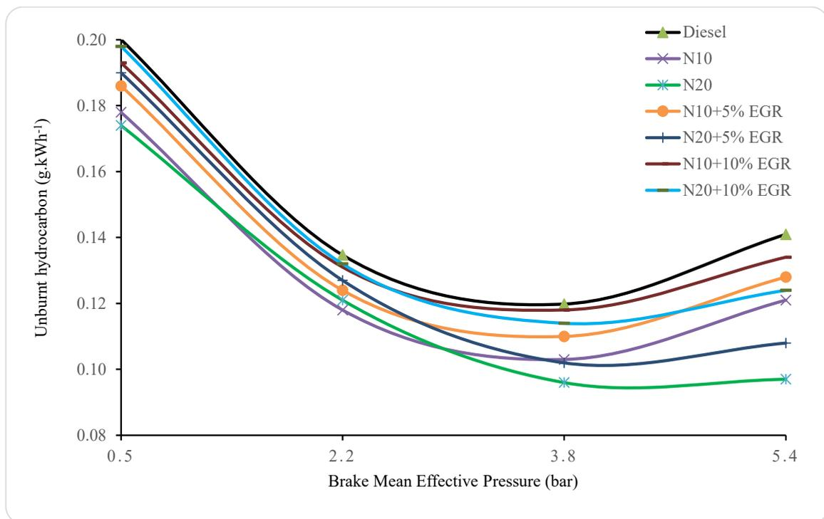
Fig. 7: Changes in unburnt Hydrocarbon with BMEP.
