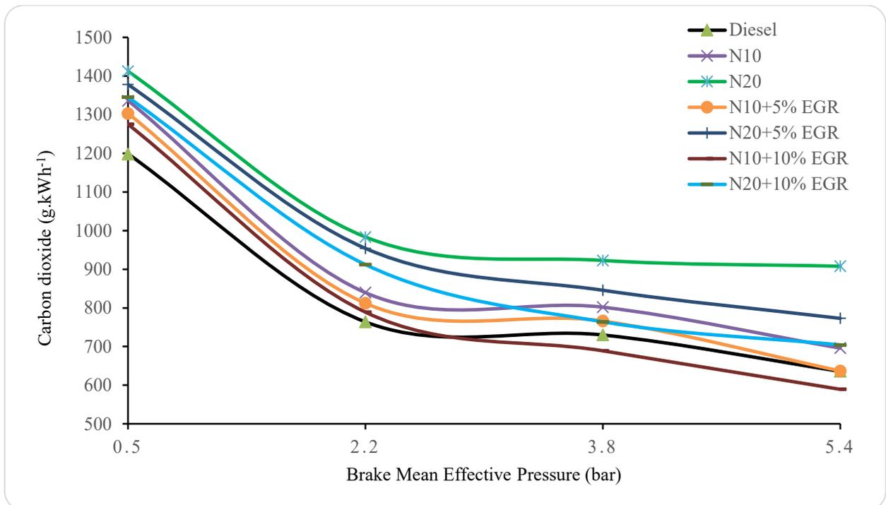
Fig 8: Changes in carbon dioxide with BMEP.
