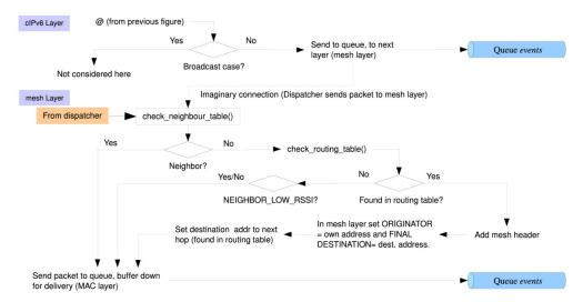
Figure 14: cIPv6 and mesh layers in the stack: BUFFER\_DOWN case
