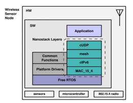
Figure 1: Relative view of Nanostack Layering in HW
