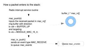
Figure 9: Details of packet entering to the stack
