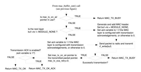
Figure 12: Details of function *mac\_buffer\_out()*
