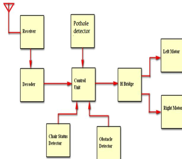
Figure:2 Receiver section
