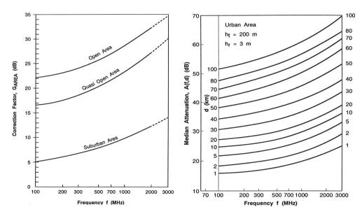
Figure 1: Median attenuation factor for Okumura Model
