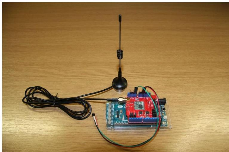
Figure 8. Arduino Due with Dragino LoRa shield and antenna
