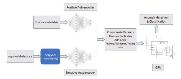
Figure 4. The proposed model architecture with SeqGAN for oversampling log messages, two Autoencoder networks, and a GRU network for anomaly detection and classification.
