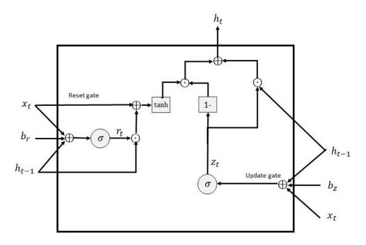
Figure 2. A GRU block with reset gate, update gate, and tangent hyperbolic and sigmoid activation functions.
