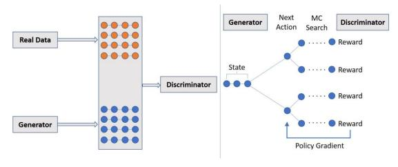
Figure 3. The SeqGAN architecture. The Discriminator on the left is trained with real data and data is generated using the Generator. The Generator on the right is trained using the policy gradient. The reward is computed by the Discriminator and this is used to determine the intermediate action values for the MC search.
