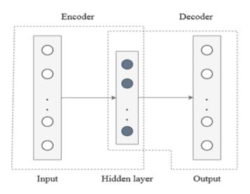
Figure 1. Autoencoder architecture with an input layer, a hidden layer, and an output layer.
