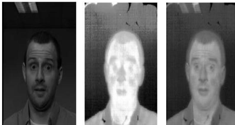
Fig 5. visible image (a), thermal IR image (b), fused image (c) [14].
