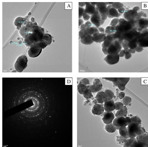
Figure 3: TEM images (A, B, C) of Ag nanoparticles (AgNPs) in low and high magnification, (D) SAED patterns of the silver nanoparticles.<sup>7</sup>
