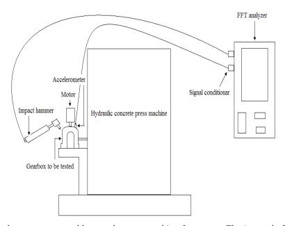
A gearbox developed a resonance problem at the gear meshing frequency. The input shaft speed is 1440 RPM and there are 38 numbers of teeth on the input pinion.
