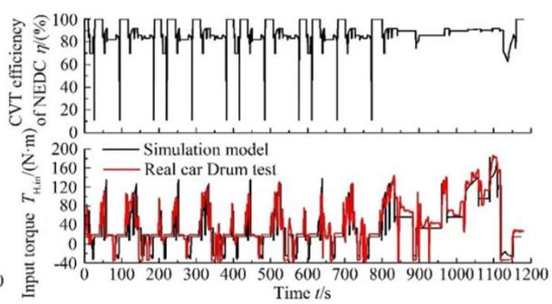
Fig. 5. Simulation results of EUDC(a)
