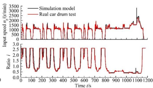
Fig. 6. Simulation results of EUDC(b)
