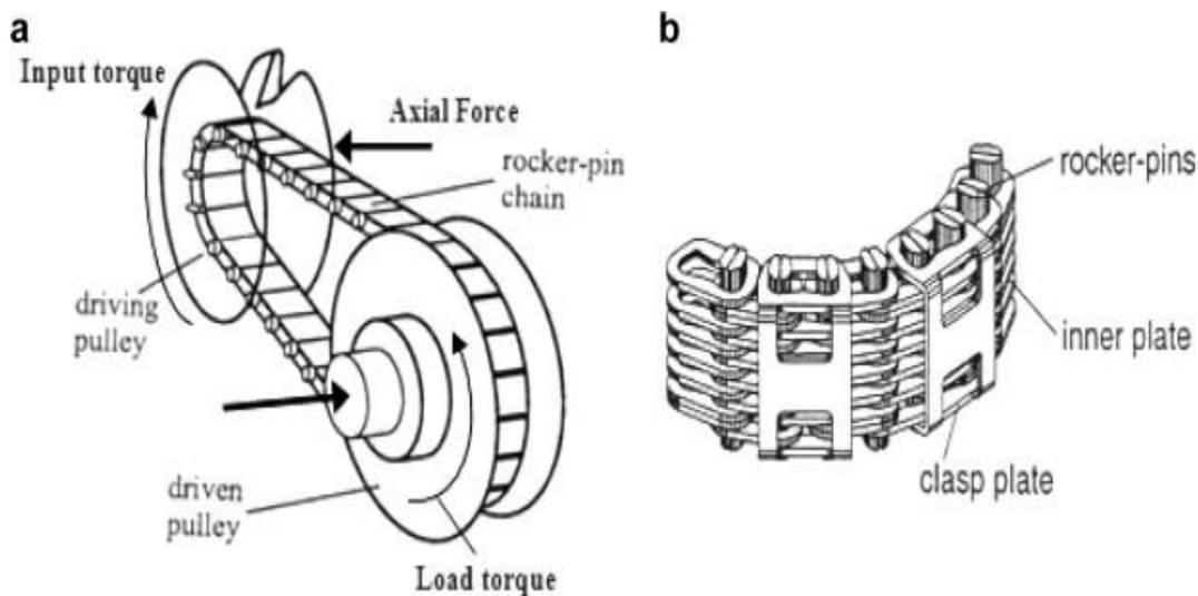
Figure 1: CVT Chain Drive. (a) basic configuration; (b) chain structure
