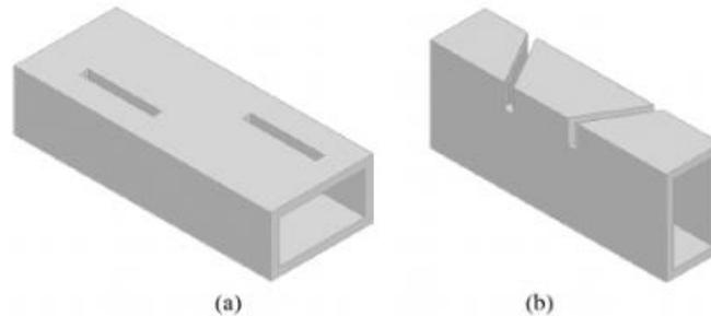
**Fig. 1.** Two types of radiating slots: (a) etched on the wide-wall; (b) etched on the narrow-wall.
