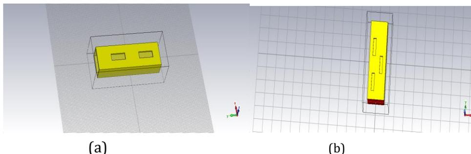
**Fig 3:-** Antenna Design. (a) two similar size lengths of slots milled on a WR90 at a similar distance from centre and aligned in a line. (b) two similar size lengths of slots milled on aWR90 at a similar distance from centre but are in zig-zag direction from each other.
