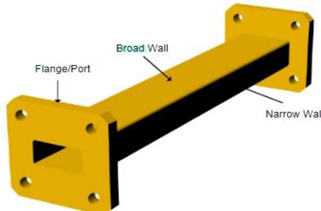
**Fig 2:-** waveguide
