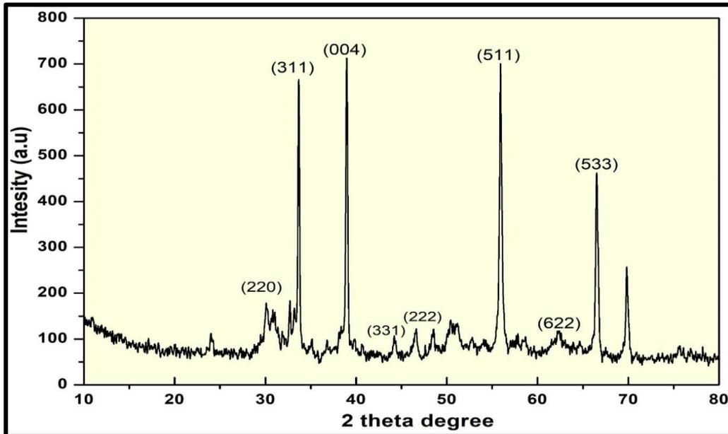
Figure 3.1: XRD patterns of CdFe<sub>2</sub>O<sub>4</sub> NPs prepared by solution combustion technique.
