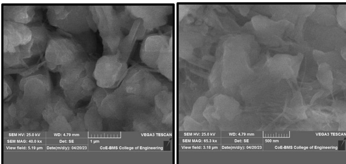
Figure 3.2: SEM micrograph of CdFe<sub>2</sub>O<sub>4</sub> nanoparticle synthesized by the impact of bio-fuel in combustion process.
