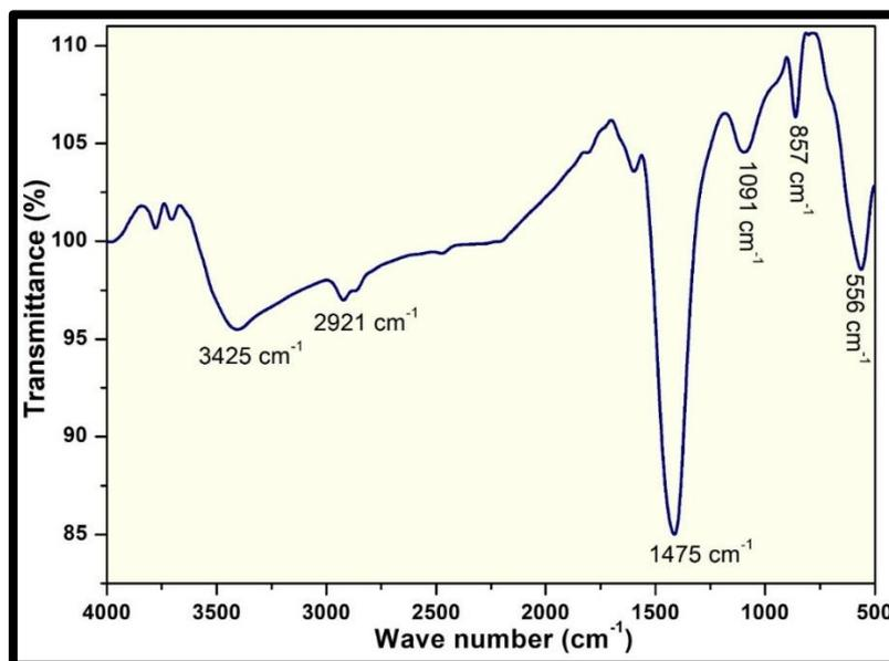
Figure 3.4: FT-IR spectra of CdFe<sub>2</sub>O<sub>4</sub> nanoparticle synthesized by the impact of bio-fuel in combustion process.
