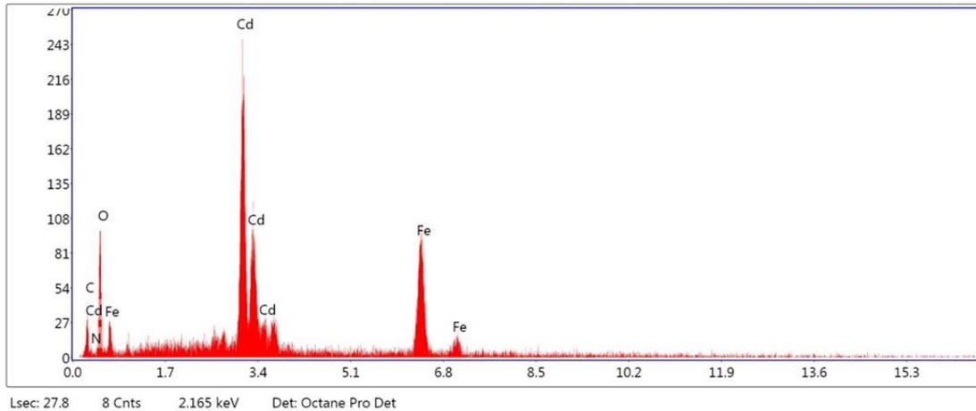
Figure 3.3: EDAX of CdFe<sub>2</sub>O<sub>4</sub> (Cadmium Ferrite) nanoparticles
