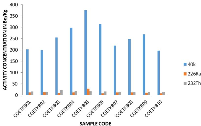
**Figure 5:** Activity Concentration of  $^{226}\text{Ra}$   $^{232}\text{Th}$  and  $^{40}\text{k}$  against sample Code
