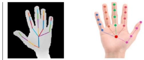
In capturing hand shape and pose, landmark detection plays a vital role. Using the Media Pipe library, this project identifies key hand key points, which serve as the foundation for feature extraction. Feature vectors are composed of distances between key points and angles formed by fingers. These vectors are then fed into machine learning models, enabling gesture classification.
