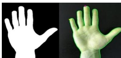
The Haar-Training algorithm is employed at this stage, which requires data samples for effective object detection. Two types of data are used: positive data, featuring clearly visible and accurately cropped hands, and negative data, where hands are not distinct, and there are no objects in the captured images.
