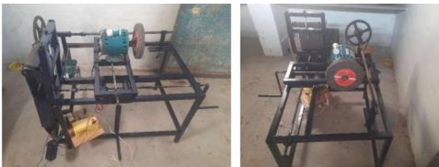
**Fig 2:** Mini abrasive belt grinding machine
