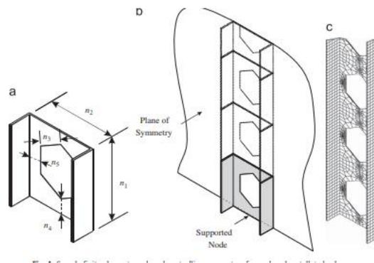
**Figure 1:** Sample finite element mesh and controlling parameters for analyzed castellated
