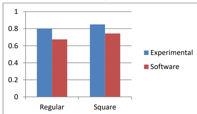
**Graph 3:** Total Deformation for regular and Square- Experimental and Software results comparison
