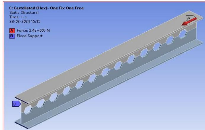
Figure 5: Loading on Column
