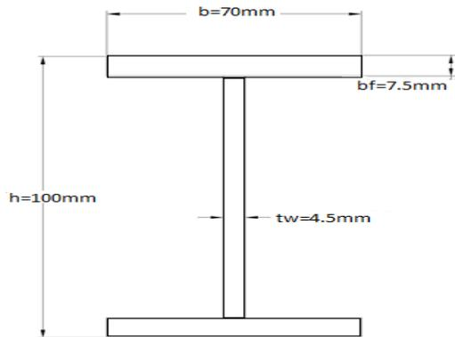
**Figure 2:** Dimension of original section
