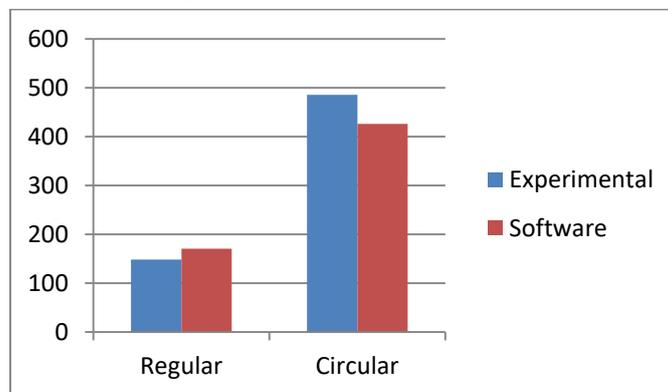
**Graph 5:** Equivalent Stress for regular and Circular- Experimental and Software results comparison
