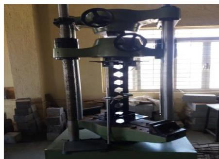
Figure 13: Testing of catellated section
