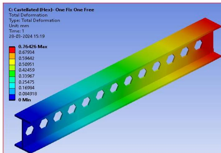
Figure 6: Total deformation
