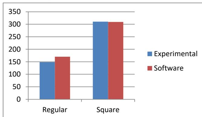
**Graph 6:** Equivalent Stress for regular and Square- Experimental and Software results comparison
