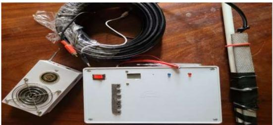
Figure 8: Designed and built FM transmitter and Receiver
