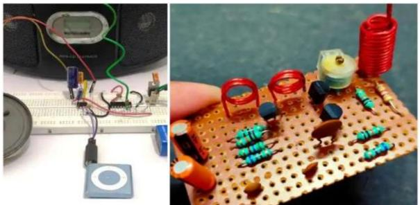
Figure 3: FM Transmitter Designed Board
