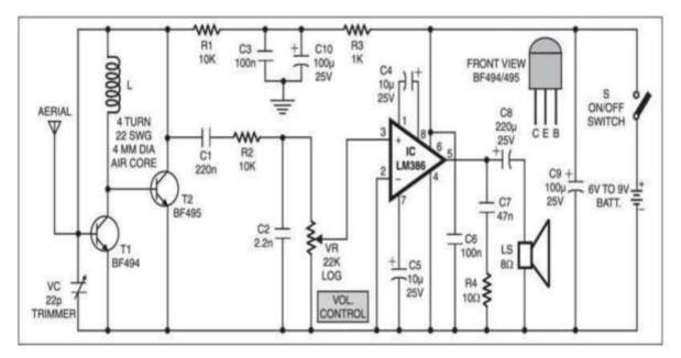
Figure 4: FM Receiver Circuit Diagram
