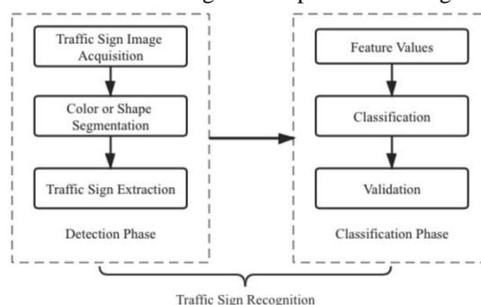
**Figure 1:** The workflow of traffic-sign Recognition.
