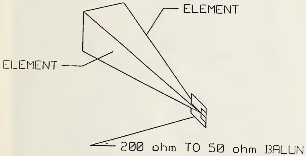
Figure 3. Balanced TEM horn antenna drawings.
