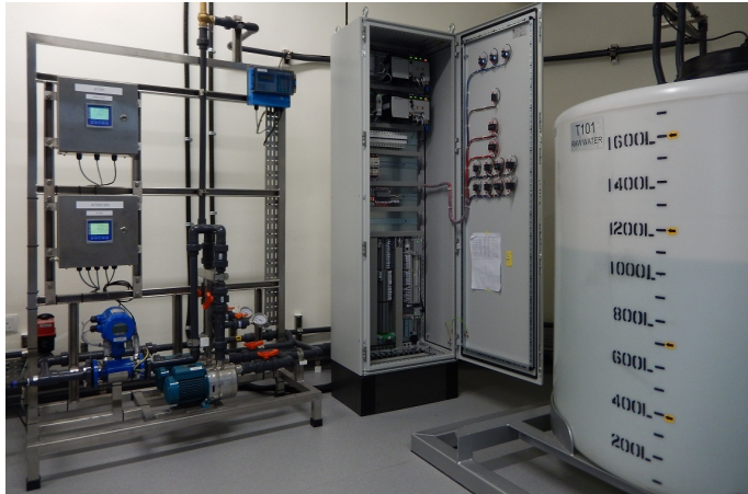
Figure 11. Testbed's Raw Water stage with two redundant PLCs (which can be seen on the top part of the cabinet), EtherNet/IP ring, pump, and water tank.
