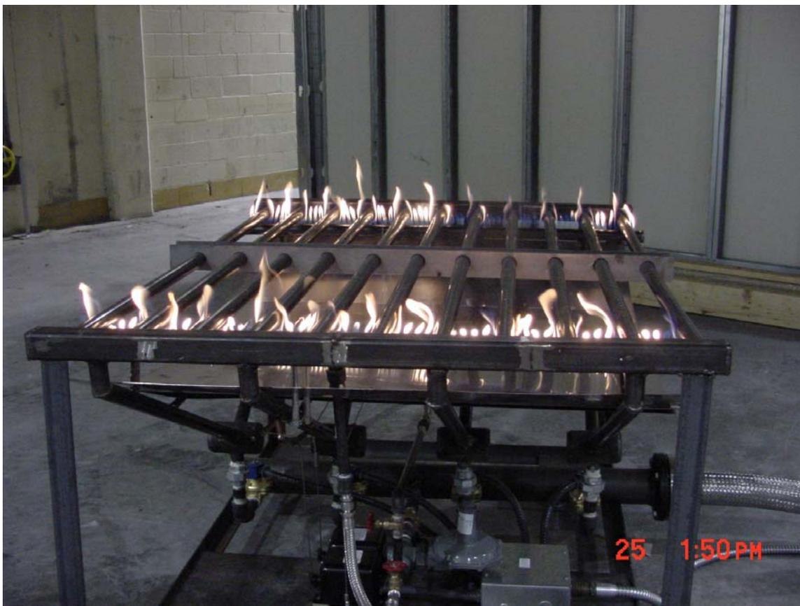
**Figure 1 Ignition of pilot tubes during start-up.**
