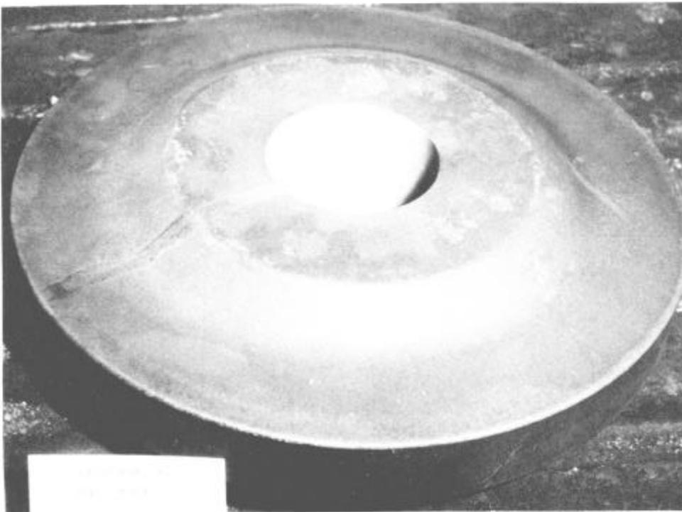
Figure 4: Rene' 95 Full-Scale Forging Preform and Jet Engine Disk Forging.
