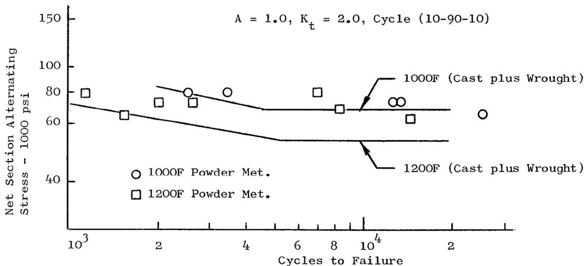
Figure 10: Sustained Peak Low-Cycle Fatigue (SPLCF) Properties of Full Scale (2.5 inch thick rim) Rene' 95 Disks.
