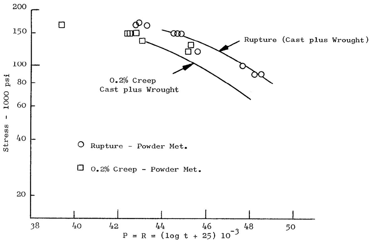
Figure 9: Creep Rupture Properties of Full Scale (2.5 inch thick rim) Rene' 95 Disks.
