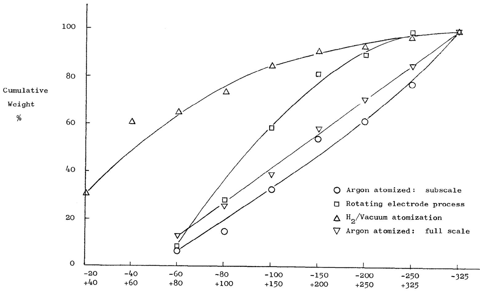
Figure 1: Particle size distribution for three subscale powder lots and average of full-scale pow
