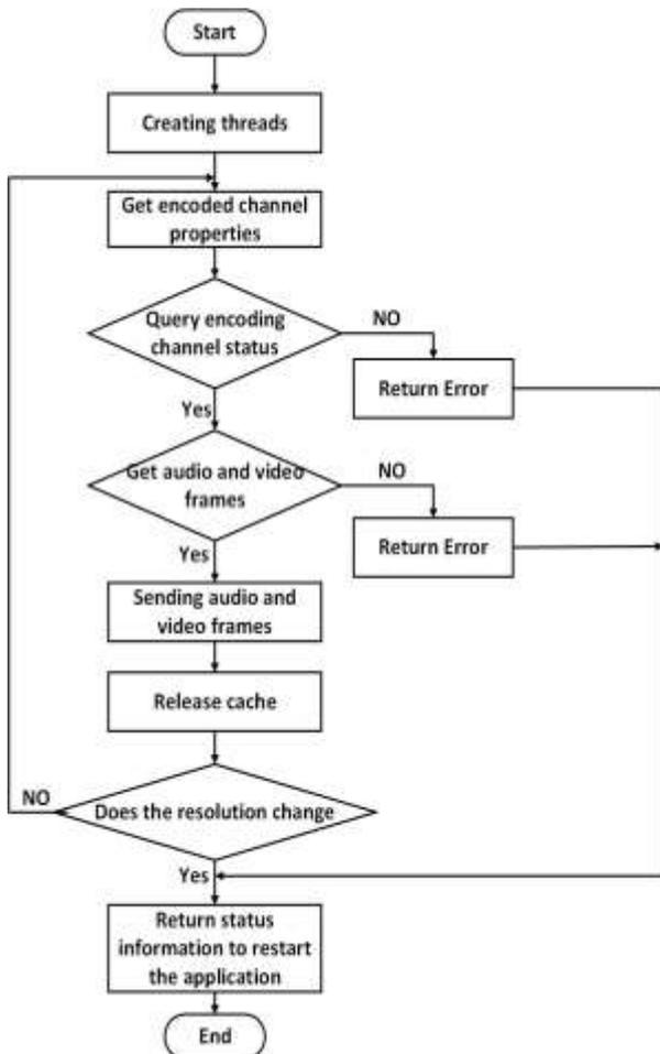
Figure 5. Flow chart of sending data interaction
